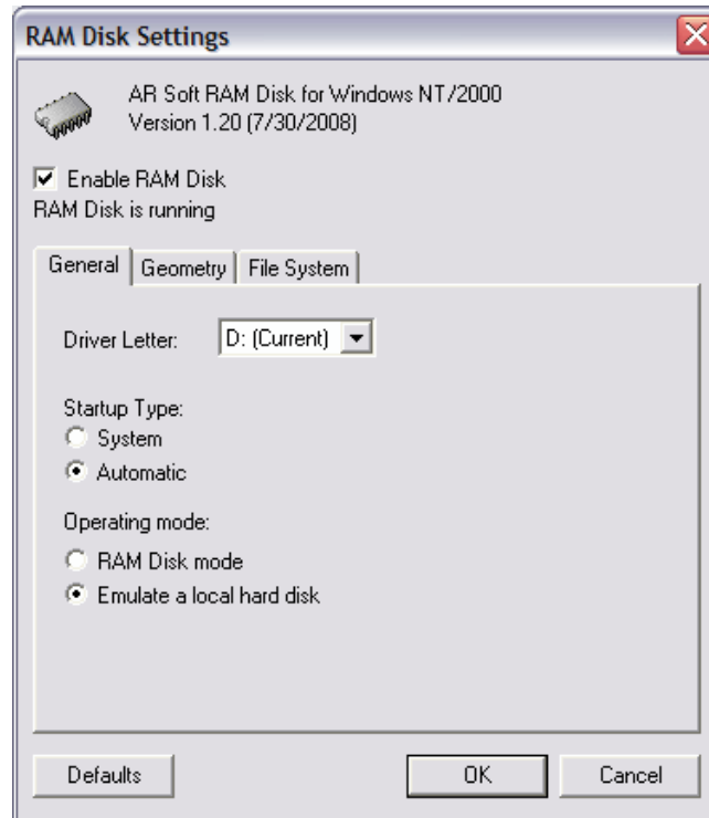
Figure 3-24 RAM Disk Configuration
