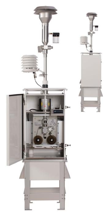
The BAM 1022 has US-EPA designation for PM<sub>2.5</sub> (EQPM-1013-209) for which a dedicated hourly output channel is available. A second, real-time output channel will provide the user with continuous PM updates down to 1-minute time resolution. The BAM 1022 is ideal for the following applications:
